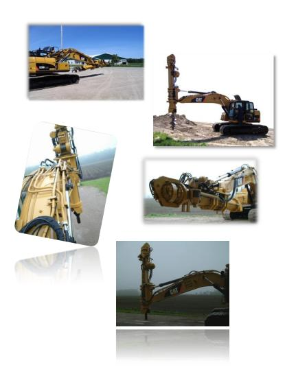
The 5033 drill attachment is used for drilling up to 33 feet deep and 9 feet wide. It can be installed on larger machines such as the CAT320DLRR. This drill operates at a torque of 50, 000 ft. lbs, and can be modified to suit your personal requirements.
